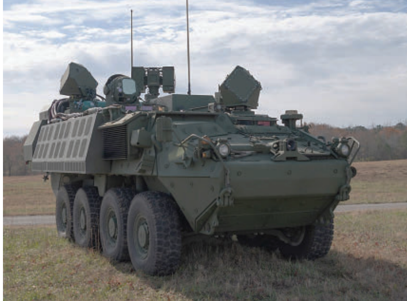
▲ The DE M-SHORAD integrates a 50-kilowatt class high-energy laser weapon system with the mobility and versatility of the Stryker A1 8x8 armored vehicle.
