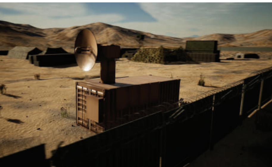
▲ An artist rendering of the Air Force Research Laboratory's Tactical High-power Operational Responder, or THOR. The technology is a portable counter-UAS system, capable of destroying swarms of drones at long range. Air Force image.
